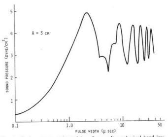
Fig. 4. Peak pressure generated in a 3-cm-radius spherical head irradiated with 2450-MHz radiation as a function of the incident pulsewidth. See Fig. 3 for other parameters.
